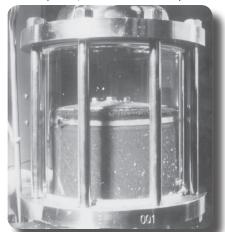
During the filtration mode, the incoming iron and manganese particles are captured by the filter media (as shown above). The filter media is comprised of synthetic fibers that are compressed and twisted into a high density matrix during the filtration cycle. The fibers capture iron and manganese particles in the feedstream through high efficiency depth filtration.
