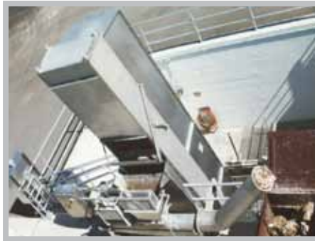
Above: Vertical Mark CI™ with full enclosure discharging into a Schloss™ Hydraulic Ram Press. At right: Three Mark CI™ Screens serve a large plant in the Middle East.
