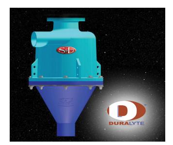
The new **PISTA® DURALYTE®** with its proprietary cone bottom delivers superior grit concentrator performance. Achieving greater than 95 percent removal of residual organic material (up to 500 GPM/32 lps), the two-piece **PISTA® DURALYTE®** also significantly minimizes wear from heavy grit loads, which delivers extended service life, and makes handling easy.
