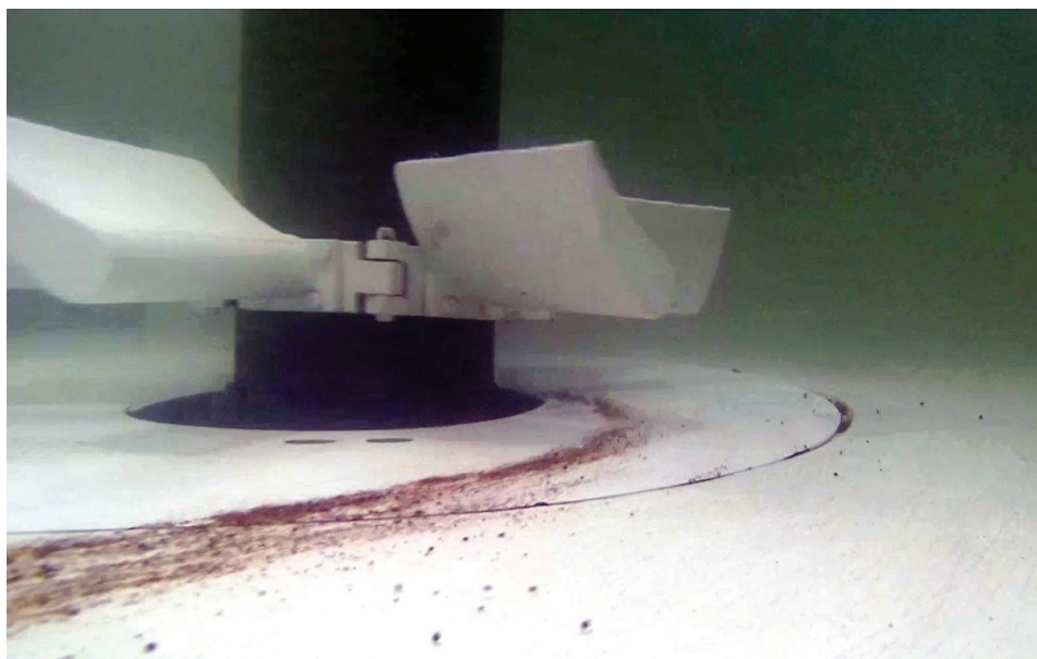
Underwater Image Of Grit Moving Along Flat-Floor Forced Vortex Grit Chamber
